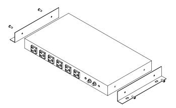
With a 5/16" nut driver, unfasten the set of 10-32 Hex head machine screws on each side of JPDU-A. Take one of the rear mounting brackets and align each side hole with the side hole on JPDU-A. Attach one rear mounting bracket using two of the unfastened 10-32 Hex screws. Repeat installations steps for the other rear mounting bracket as shown above.
