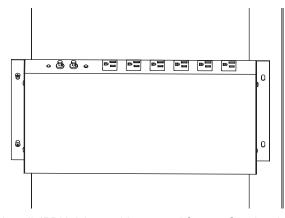
Install JPDU-A in a cabinet or 19" [483mm] rack using appropriate hardware (not provided) for mounting.
