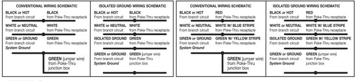
WARNING: Ground wire from junction box must be connected to system ground.
