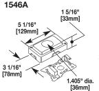
Single Receptacle Box - Accommodates commercially available straight blade and locking single receptacles with face diameters of 1.38-1.40" [34.5-35mm]. Base has 1/2" [12.7mm] and 3/4" [19mm] trade size concentric KOs. Cover has 1500 and 2600 twistouts on all four sides. Two 1500WC wire clips included.
