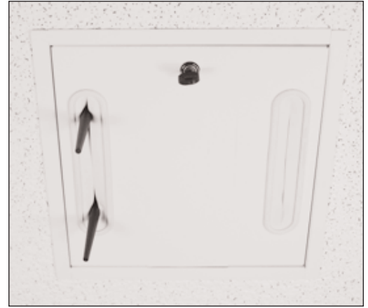
Wireless Access Point Ceiling Enclosure installed in ceiling tile. The cover contains knockouts to support a variety of antenna configurations and installable grommets that protect the interior of the enclosure from dust and debris.
