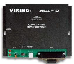
The **PF-6A** power failure bypass system makes it possible to receive calls during phone system and power outages. The **PF-6A** bypass unit connects 6 pre-assigned single line station phones directly to user-assigned C.O. trunks. A built-in ground start converter permits outbound calls from standard phones.
