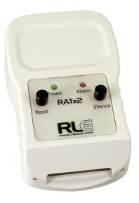
he Raptor RA1x2 is a relay splitter and alarm annunciator. It can split a single dry contact relay input into two electrically isolated outputs and annunciate the change in state of any dry contact relay signal.
