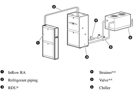
Note: Install isolation valves and particulate strainers with 20 mesh stainless steel screen (opening size = 865 micron) in the supply line between the chiller and RDU. For more information, see the RDU Installation Manual. \*The RDU is a required unit available through APC. For more information, see the RDU Technical Data Manual. \*\*Piping between the chiller and the RDU will vary based on local codes and site conditions.
