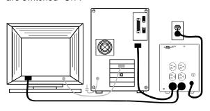
Caution: Do not connect a laser printer to the Battery Backup Outlets.
