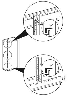
4. When the vertical mounting flange is in the proper location, slide each screw up until the teeth in the bracket engage fully with the teeth in the side brace, and tighten the screws.
