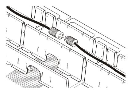
Connect each of the three receptacles on the multi-branch cordset adapter to a different APC Rack PDU. See the tables beginning on the previous page for compatible APC Rack PDUs.
