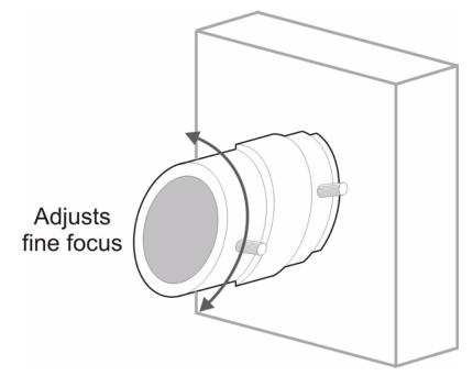
**Note:** If you are unable to get the image into focus you may need to readjust the Wide-Angle / Telephoto Adjustment Ring, then try adjusting the Fine Focus ring again.
