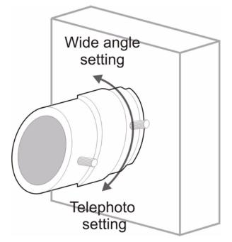
5. Loosen (but do not completely unscrew and remove) the locking screw on the Fine Focus Ring. Then, while referring to the image that is displayed in the Basic or Advanced View, make small adjustments to the position of the Fine Focus Ring until you are satisfied with the image that is displayed in the Basic or Advanced View. Then, tighten the locking screws on the Fine Focus Ring and the Wide-Angle / Telephoto Adjustment Ring to lock them in place.
