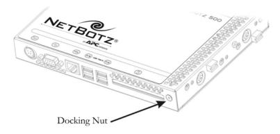
Loosen the nut until the docking indicator can be seen in the upper windo was shown below.
