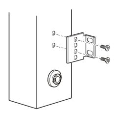
2. Install the Rack PDU on a vertical mounting rail in your rack or enclosure.
