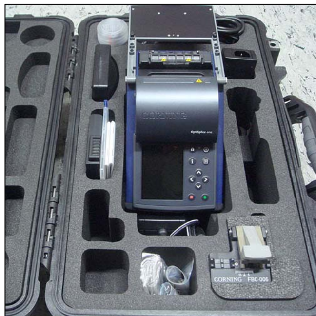
OptiSplice one operational in Transport / Workstation case
