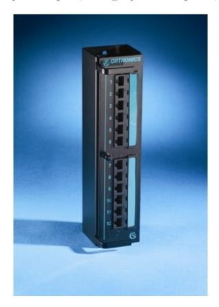
Clarity 5E 12-port mini patch panel is component compliant to EIA/TIA Category 5e performance requirements. Its high density design on hinged wall mounting provides access to wire terminations while maximizing wall space in small or confined locations. The panel measures 10" x 2.5". Jacks are grouped in sixport modules. Part of the Clarity 5E link and channel solution that provides significant installed performance headroom.
