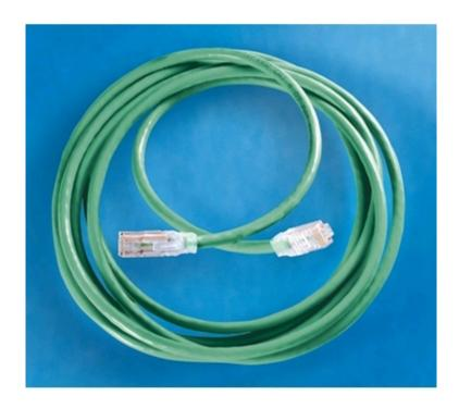
Clarity 5E Premium Category 5e Modular Patch Cord, green, 3', Category 5e, four-pair UTP stranded 24 AWG PVC/CM, center tuned with Clarity 5E connecting hardware for optimum Category 5e installed performance using Ortronics Paralign 2 pair-positioning technology
