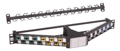
The CopperTen® Augmented Category 6 Angled Patch Panel optimizes 10 Gb/s transmission performance with offset jack positioning to counter the negative effects of alien crosstalk. The angled port design improves all aspects in managing horizontal cable and patch cables while improving density when used with Glide Cable Management. It also makes modifications easy, avoids unintended disconnects and cable damage, and protects bend radius to avoid violations that result in signal degradation.
