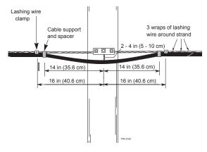
**3.18.** In general, fiber optic cable drip loops are formed by hand. Hand forming of drip loops is permissible for fiber optic cable as long as the minimum bend radius of the cable and the dimensions illustrated previously are not exceeded. Drip loops can also be formed by an expansion loop forming tool provided that the loop conforms to the specifications shown.
