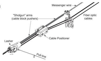
**3.28.** Corning Cable Systems recommends that as a cable run is lashed up, span-by-span, the lashing wire should be terminated at each pole with a lashing wire clamp. This practice will ensure that only one span of cable will be unsupported if a lashing wire is cut.
