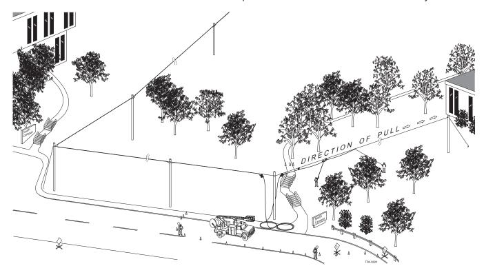
**8.5.** This last section must be lashed from the moving reel / stationary reel transition point towards the free end of the cable.
