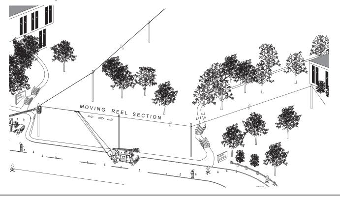
**8.4.** If the destination of the route is also inaccessible to vehicles, unreel and figure-eight the cable to gain access to the other end of the cable. Pull the cable into place beneath the strand with a stationary reel method.
