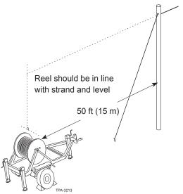
Be prepared to level the reel by means of planks or other supports under the vehicle or leveling the ground in unpaved areas. Line up the center of the cable reel with the strand as closely as possible.
