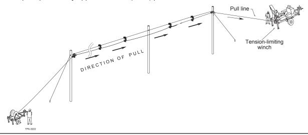
**7.20.** As with hand-pulled stationary reel installations, monitor the entire cable route during the cable pull. Station crew members equipped with two-way communications so that the entire run is under observation, making it possible to instantly stop the pull, if necessary. In addition, use a dynamometer to measure tension on all long cable pulls and short, difficult sections where pulling force might approach or violate the cable's specifications.
