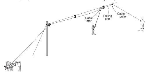
**7.13.** Continue the hand-pull, span-by-span pulling the cable along the strand and adding cable blocks for support.
