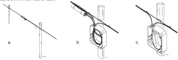
**3.39.** Corning Cable Systems recommends that splicing be done on the ground, not in an aerial bucket. Consequently, it is necessary to allow enough slack at each splice point to bring both cables to the ground and into a convenient work area, plus 16 ft (5 m).
