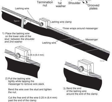
NOTE: The three wraps around the strand are necessary to reduce horizontal stress caused by friction between the lashing wire and the strand. The wraps also prevent kinking in the cable and broken lashing wires which result when the lashing wire termination is made without strand wraps.
