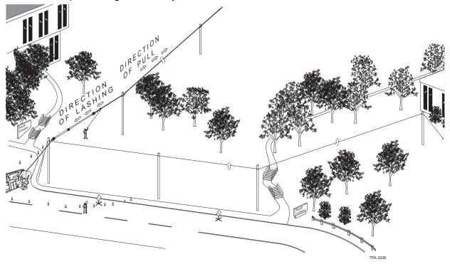
**8.3.** Following placement and lashing of this section, install the vehicle-accessible remainder of the cable route with the moving reel method.
