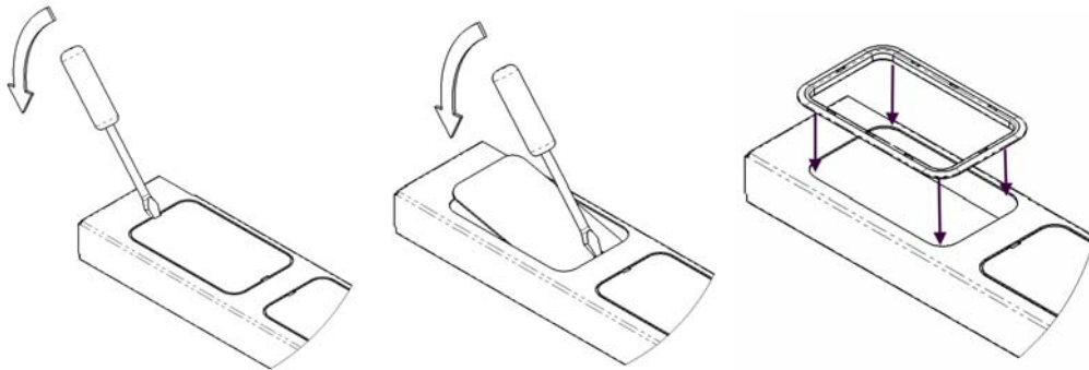
Fig. 2.5b Removing a knockout
