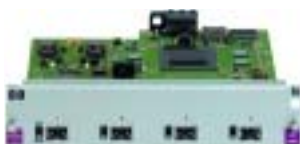
HP ProCurve Switch xl Mini-GBIC Module (J4878A) with 4 open mini-GBIC slots
